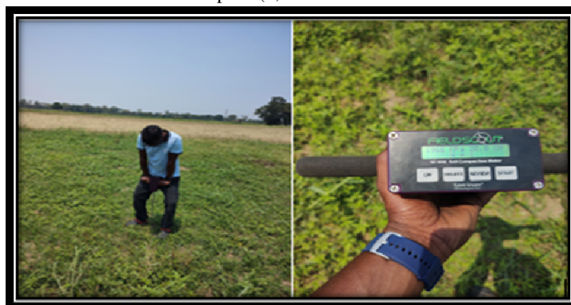
Plate 2: Measurement of cone index on field before test
