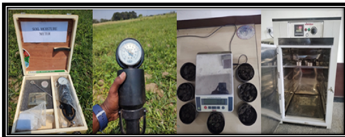
Plate 1: Methods for measurement of moisture content on actual field condition
