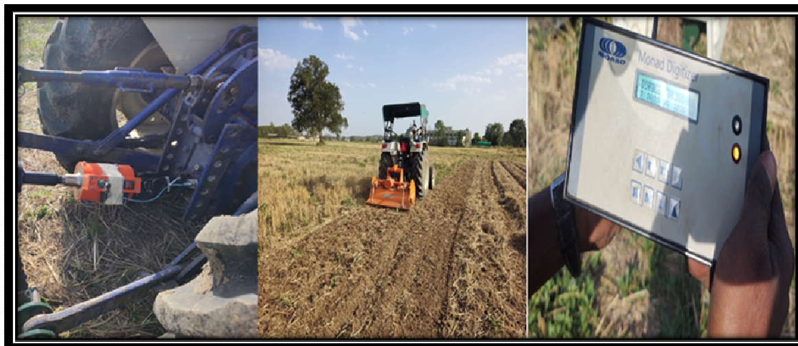
Plate 5: Measurement of torque with torque sensor
