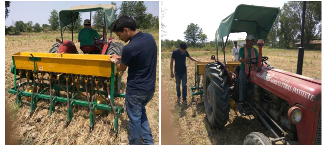
Fig. 2 : A view of sowing of wheat by eleven tyne zero till drill.
