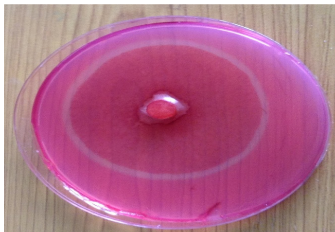
Fig. 1: Diameter of the aura of hydrolysis of the Ag 2 isolation
