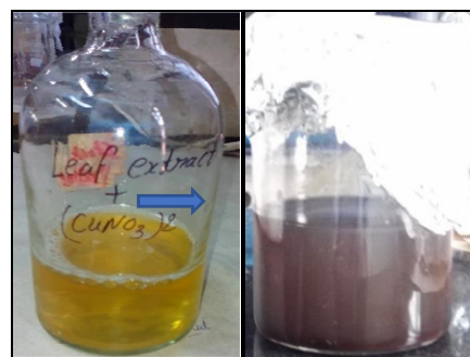
Fig. 2: The formation of Thuja nanoparticles confirmation with the change in colour of extract after addition of copper nitrate
