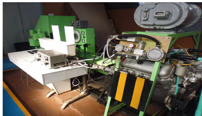
Fig. 1 : Load test bench with the YaMZ-238 engine operating on the gas-diesel cycle
