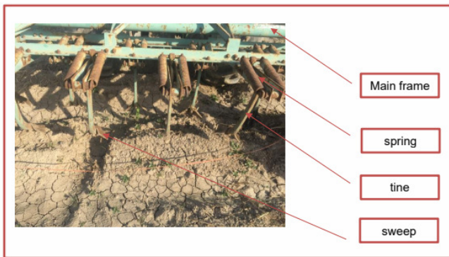
Fig. 2 : spring loaded cultivator used in the experiment
