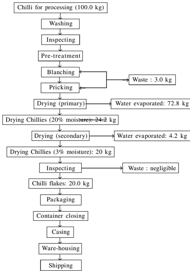
**Plate 4 :** Flow diagram for drying of chillies.
