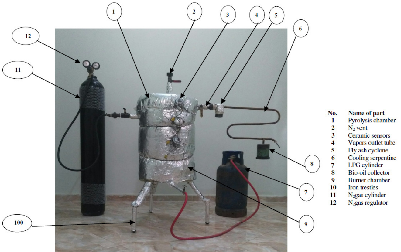
Fig. 1 : Photo of the experimental setup of the proposed fixed-bed pyrolyzer used for the co-pyrolysis of the ground MPL, SB and RS
