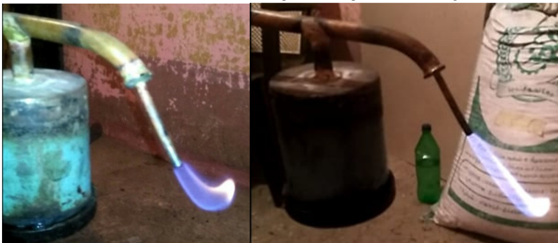
Fig. 2 : The pyrolytic gas flame from the pyrolysis process.
