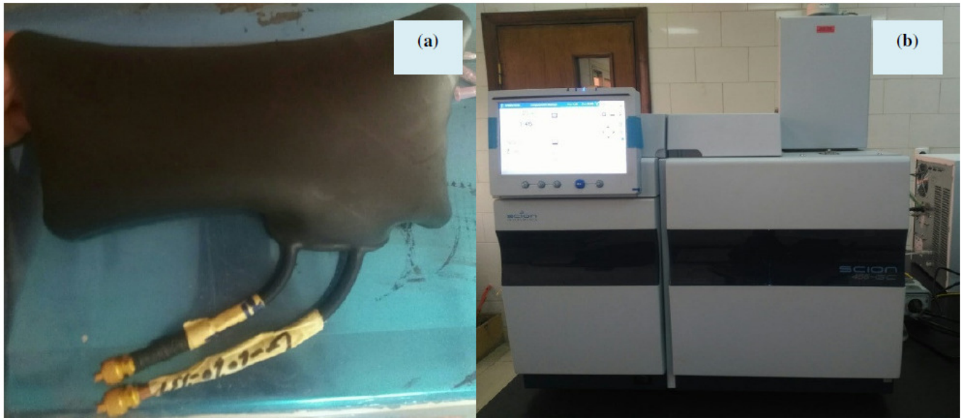
Fig. 3: The pyrolytic gas analysis: a)The rubber bladderb) the gas chromatography.
