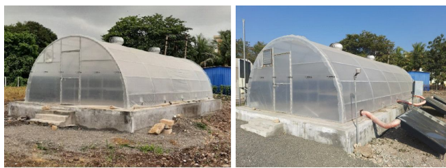
Plate 1 : Solar tunnel dryer on natural air convection mode and forced air convection mode.
