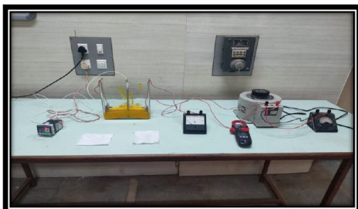
Fig. 10 : Ohmic Heating Setup.
