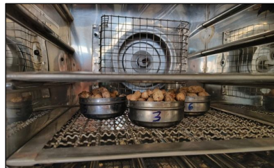
Fig. 4 : Oven-drying method for determination of moisture content.
