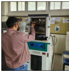
Fig. 4 : Oven-drying method for determination of moisture content.
