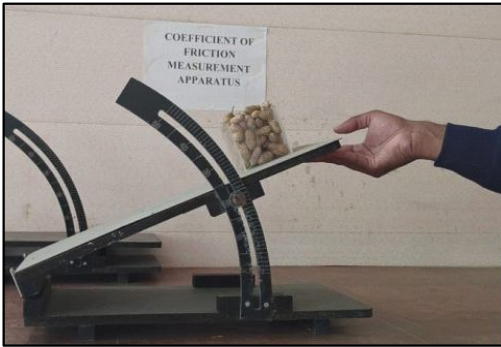
Fig. 6 : Tilting table apparatus for measurement of coefficient of friction.
