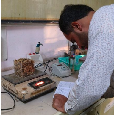
Fig. 3 : Determination of Bulk Density.
