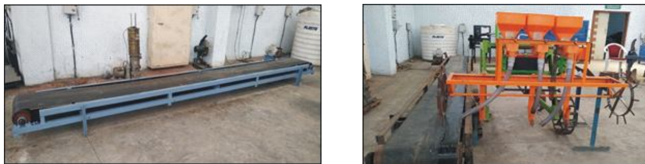
Fig. 3 : Sticky belt setup and arrangement of planter on sticky belt.
