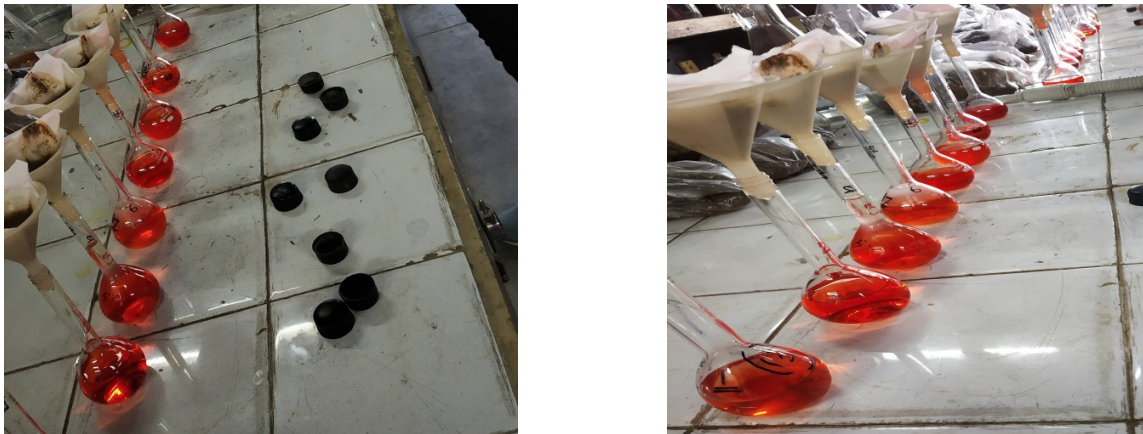
Fig. 1 : T 8 treatment samples for measuring dehydrogenase enzyme activity
