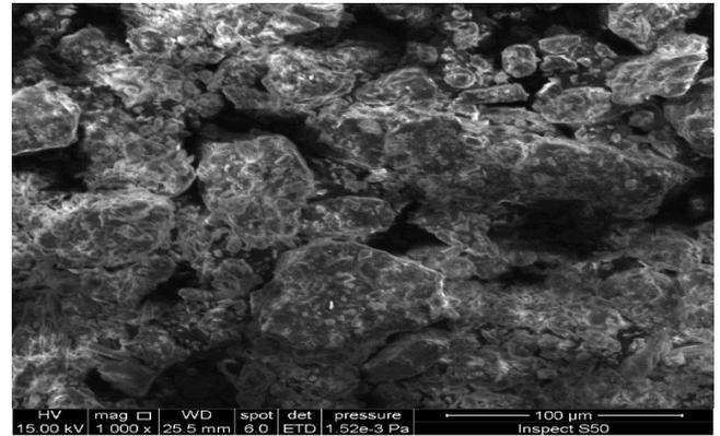
**Fig. 5 :** SEM image analyses of Soil sample of Al-Sadr City 1000 KX magnifications.
