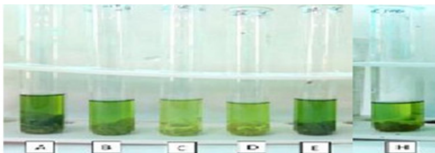
Figure 3: Effect of CR (100 mg/L) (laboratory scale treated) on chlorophyll content; A-Control, B-Untreated, C-Unmodified WB treated (1st cycle), D-Unmodified WB treated (2nd cycle), E- Unmodified WB treated (3rd cycle), H-Organism treated.
