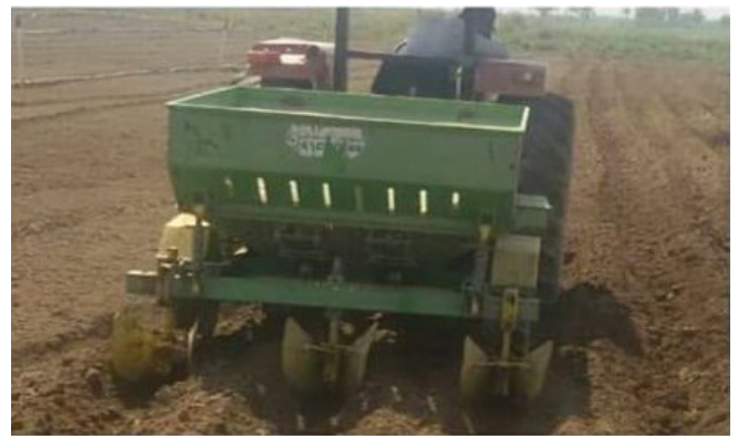
Fig. 2 : The machine (type Adwhit) used for potato planting .
