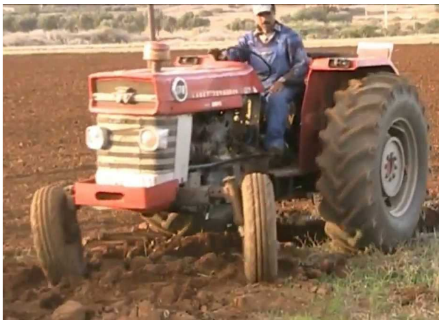
Fig. 1: The tractor (type FIAT-1880DT) with a moldboard plow, used for soil tillage.
