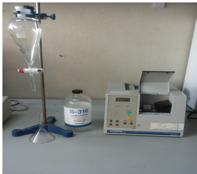
Fig. 4 : HORIBA oil content analyzer used to detect organic pollutants (hydrocarbons).
