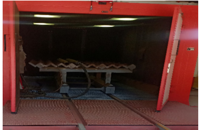
Fig. 2: blasting of tubing with lance unit
