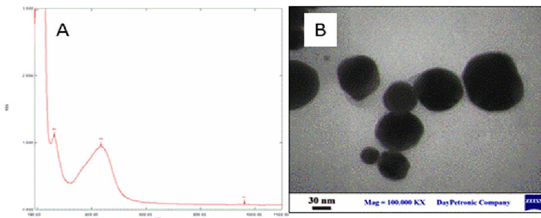
**Fig. 2:** A: Cr-AgNPs plasmon peak at 434.50 nm.; B: TEM image of Cr-AgNPs with the average size of 30 nm.
