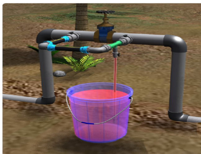
Fig. 1 : Venturi Meter (Source - Jain Irrigation Systems Limited)
