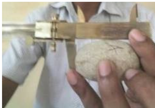
Fig. 2: Vernier calliper measuring device for cocoon measurement.
