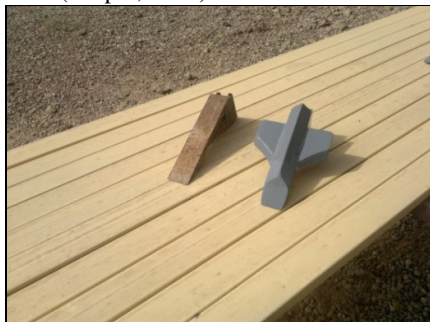
Fig. 7 : Modified tine at right and Conventional tine at left of the image
