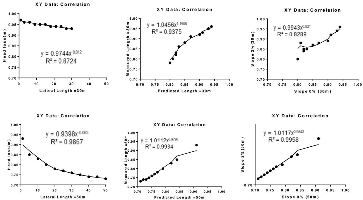
Fig. 7 : Correlation coefficient of onset sprinkler irrigation system for different sprinkler lines lengths
