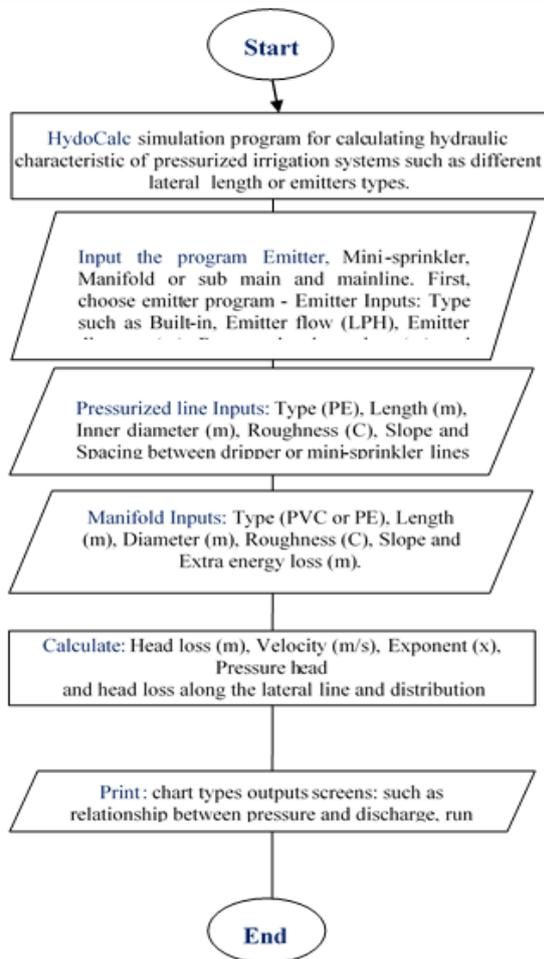
**Fig.1:** Flow chart components of HydroCalc simulation Program for planning, design, and calculating the hydraulic analysis of drip and sprinkler irrigation systems at different slopes or levels
