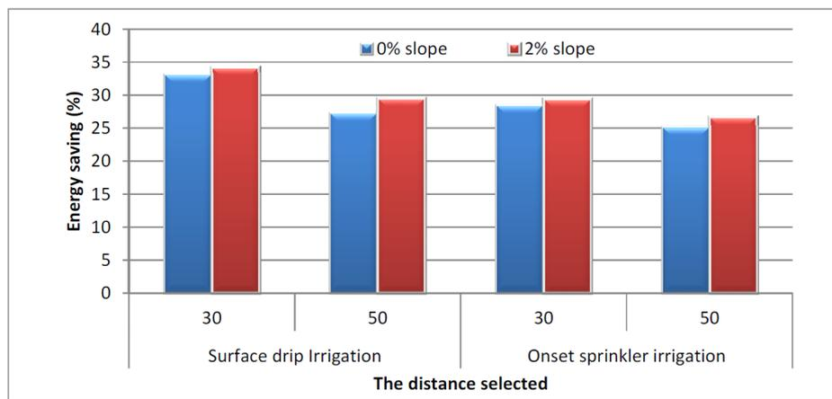
Fig. 8 : Energy saved closed circuit designs
