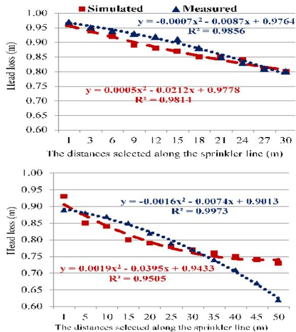
Fig. 5: Simulated and measured head losses with operating at a line pressure of 1.0 bar, 2% slope under the solid-set sprinkler irrigation design
