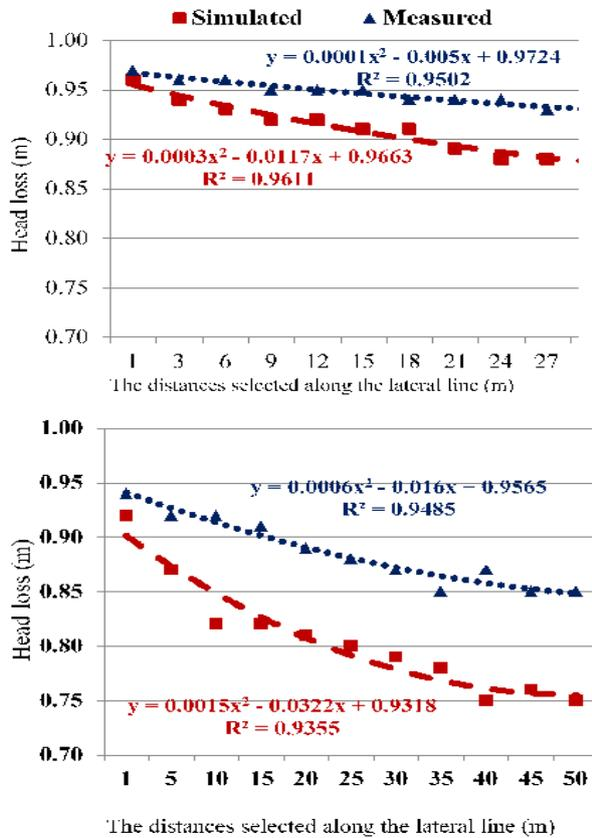
Fig. 2: Simulated and measured head losses with operating at a line pressure of 1.0 bar, 0% slope under the surface drip irrigation design
