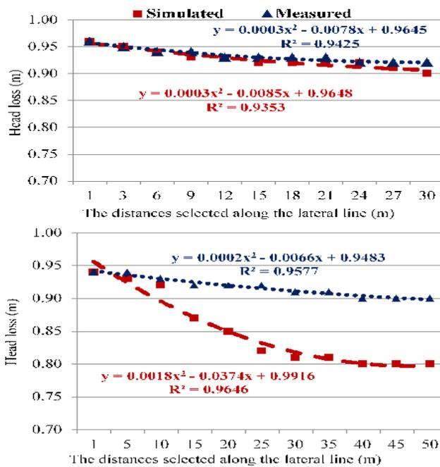
Fig. 4: Simulated and measured head losses with operating at a line pressure of 1.0 bar, 2% slope under the surface drip irrigation design
