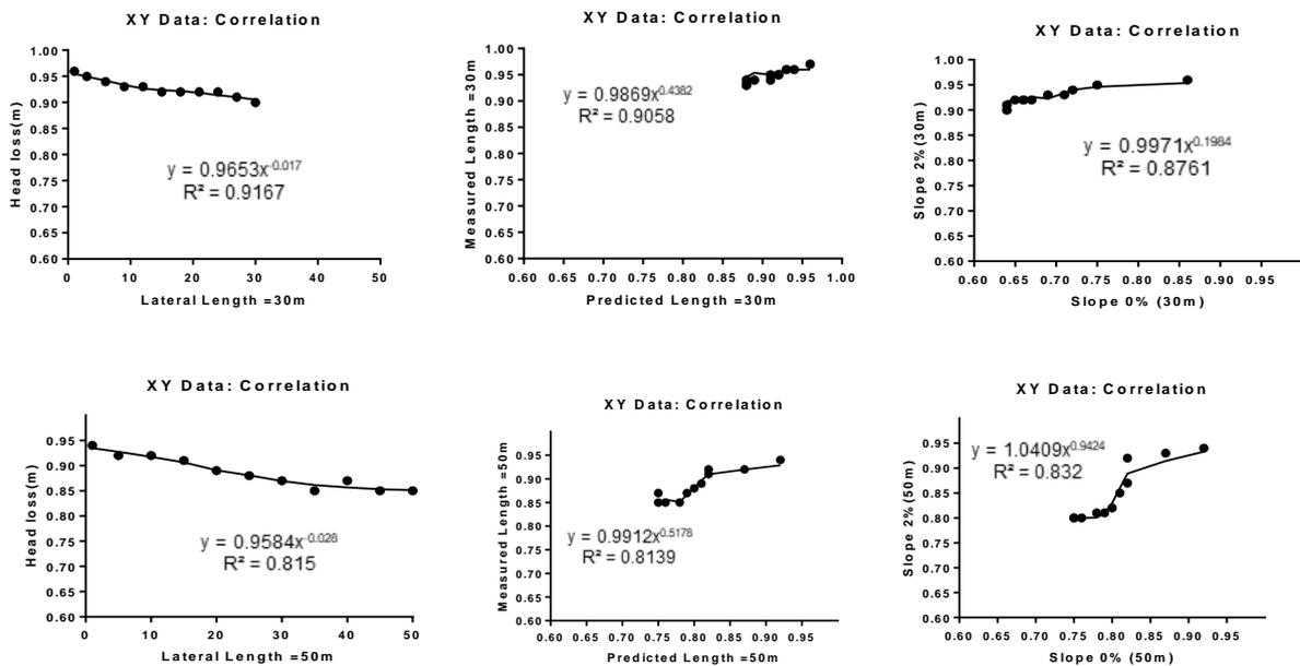
Fig. 6: Correlation coefficient of surface drip irrigation system for different dripper lines lengths
