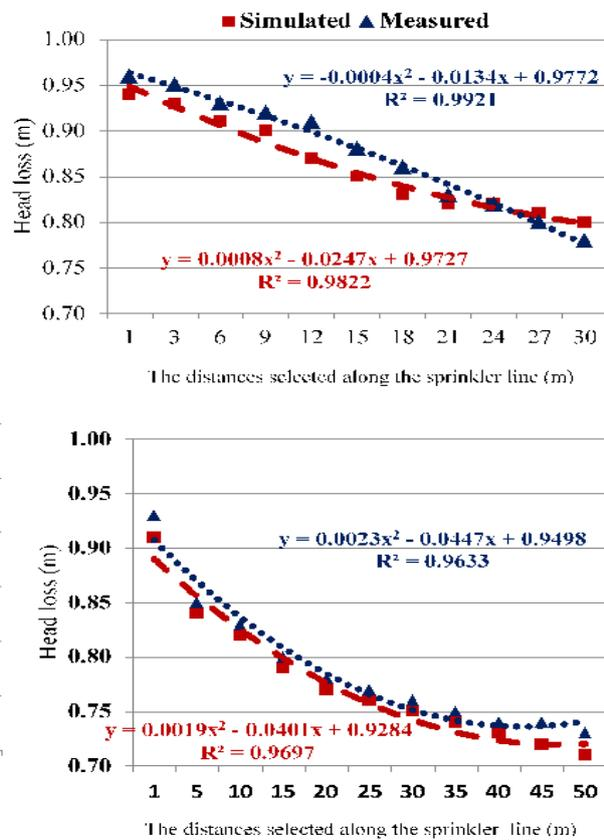
Fig. 3: Simulated and measured head losses with operating at a line pressure of 1.0 bar, 0% slope under the solid-set sprinkler irrigation design
