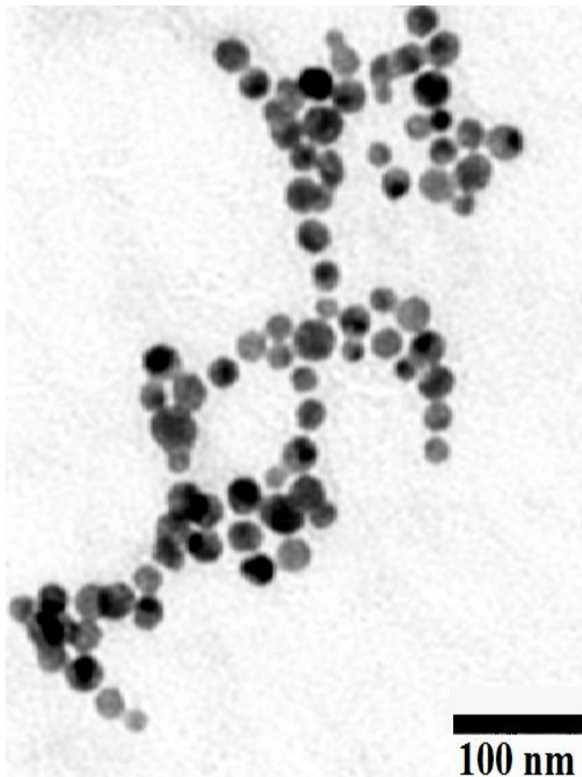
Fig. 4 : Shape of gold nanoparticles in TEM with 46000 X magnification force.
