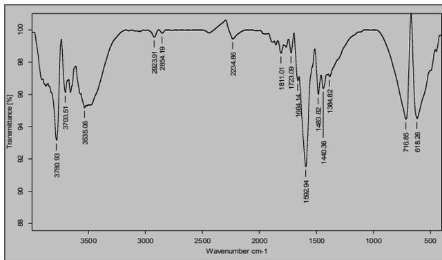
**Fig.-7:** FT-IR spectrum of colloidal silver nanoparticle suspension after bioreduction using *A. nobilis* leaf extract
