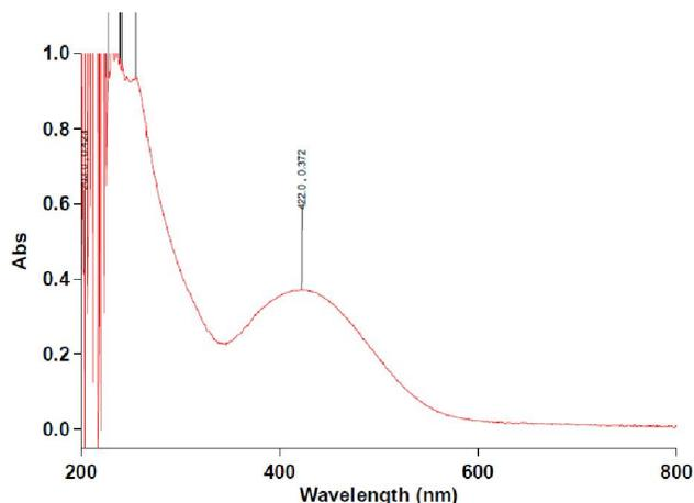
**Fig.-2:** UV-Visible spectra of silver nanoparticles synthesized by treating 1mM aqueous AgNO<sub>3</sub> solution with 5% *A.nobilis* leaves extract.
