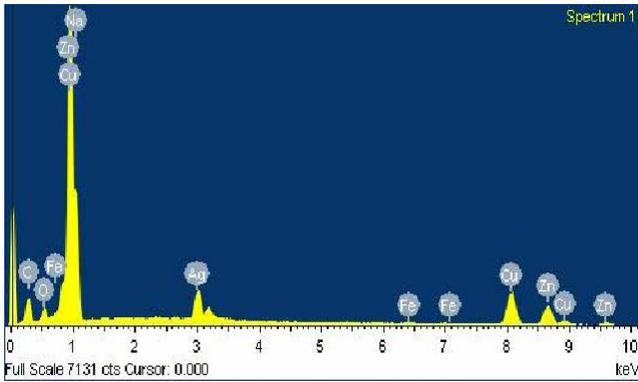
**Fig.-5:** EDAX spectrum of the silver nanoparticles synthesized using *A. nobilis* leaf extract
