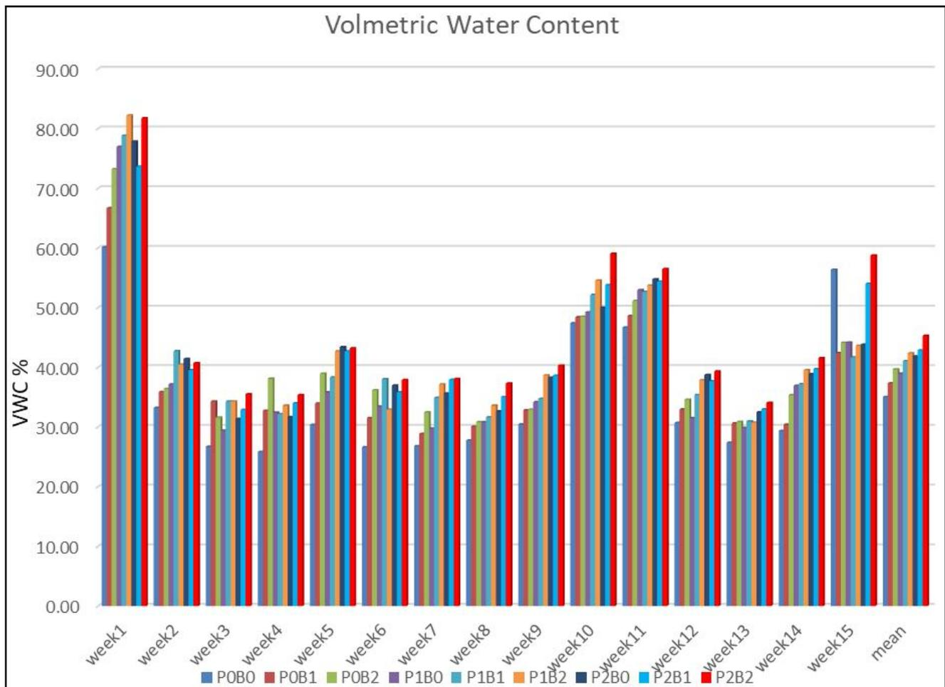
Fig. 1: The Volumetric Water Content measured by Time Domain Reflectometer TDR300.
