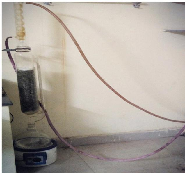
Fig. 2: Overall view of extraction using Soxhlet apparatus.
