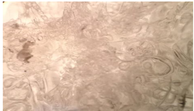
Fig. 3: Microscopic examination of the fractional section obtained in the unsaturated polystyrene sample, which was not exposed to the thermophysical treatment, as it shows that the fracture is a simple brittle fracture type. ( \times 400 )
