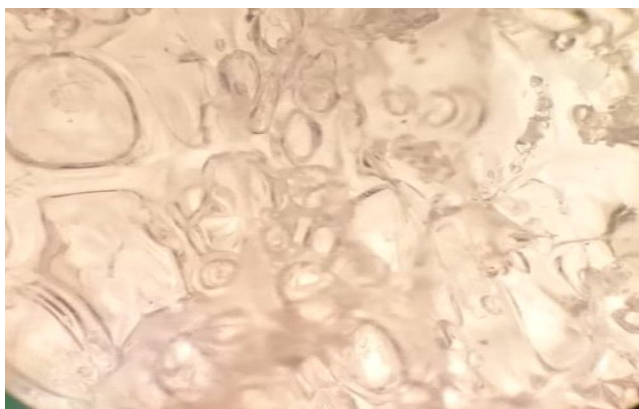
Fig. 4: Microscopic examination of the fractional section obtained in the unsaturated polystyrene sample exposed to the thermal physical effect at a temperature ( T = 100\text{ C}^\circ ) for a period of two hours shows that the fracture is of a brittle type (medium Brittle). ( \times 400 )
