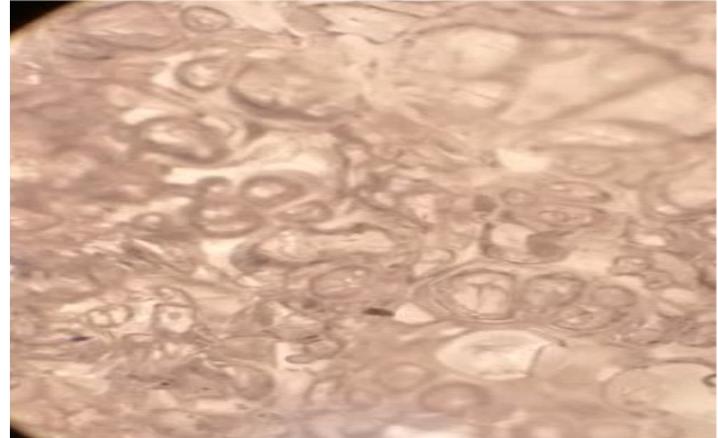
Fig. 10: Microscopic examination of the fracture section obtained in the saturated polystyrene sample exposed to the physical thermal effect at a temperature ( T = 60\text{Cp} ) for period of (4) hours. ( \times 400 )
