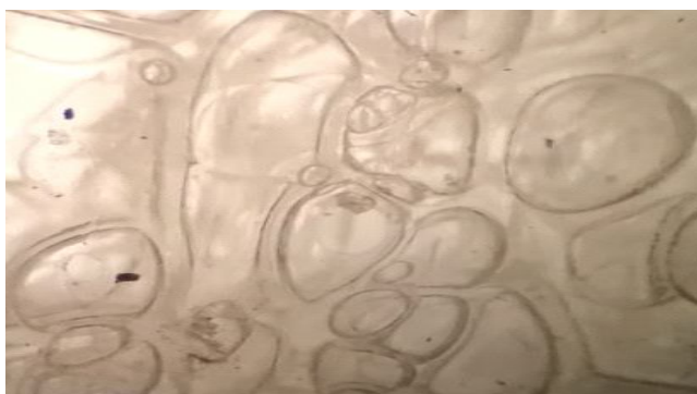
Fig. 5: Microscopic examination of the fracture section obtained in the unsaturated polystyrene sample exposed to the thermal physical effect at a temperature ( T = 100\text{ C}^\circ ) for period of (8) hours, showing that the fracture is of a brittle type (completely brittle). ( \times 400 )
