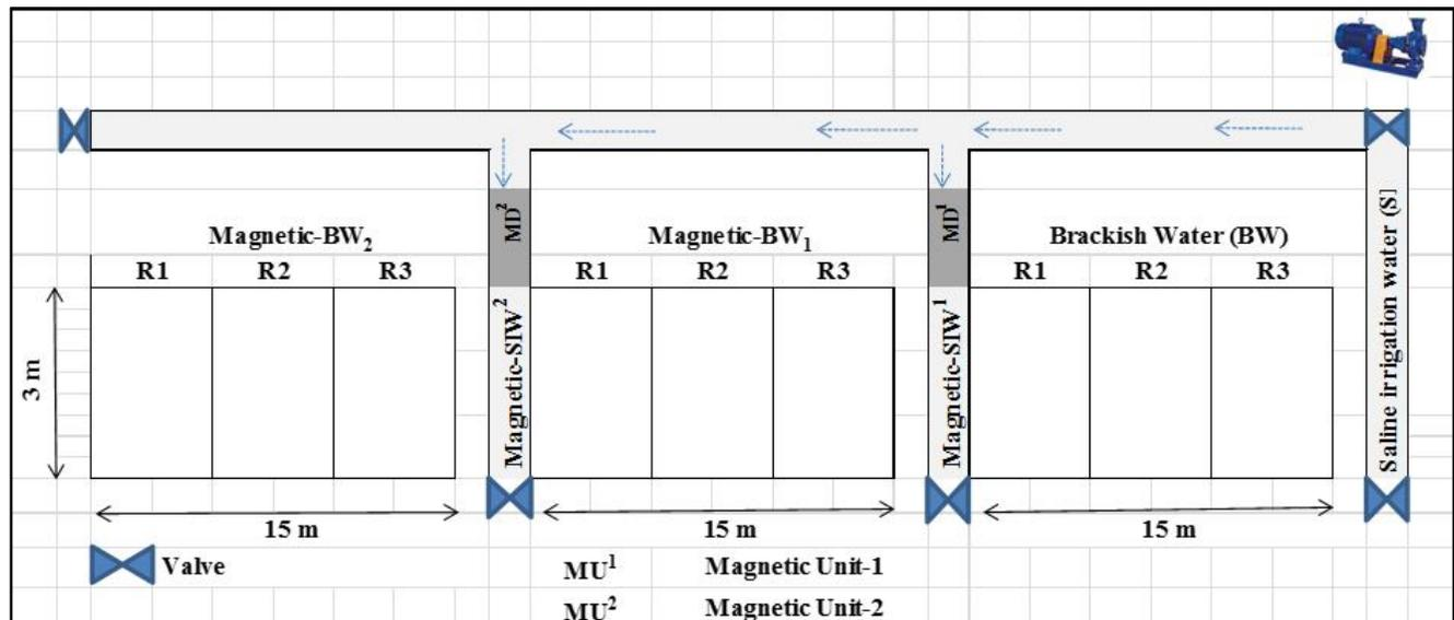
Fig. 1: Layout and design of experiment.
