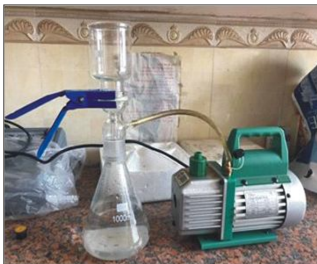
Fig. 2: Demonstrate sample filtering using a micro-fiber filter.
