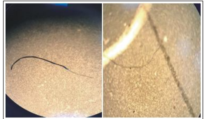
Fig. 8: Shows the shapes of the plastic particles under the optical microscope with a magnifying force of (10x).
