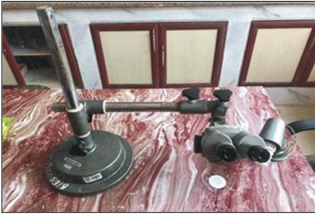
Fig. 4: Determination of plastic particles. Using an anatomical microscope from (OLYMPUS).
