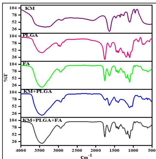
**Fig. 1:** FTIR spectra of KM (Kaempferitrin), PLGA, KM+PLGA and KM+PLGA+FA nanoparticles recorded in the range of 4000-500  $\text{cm}^{-1}$ .
