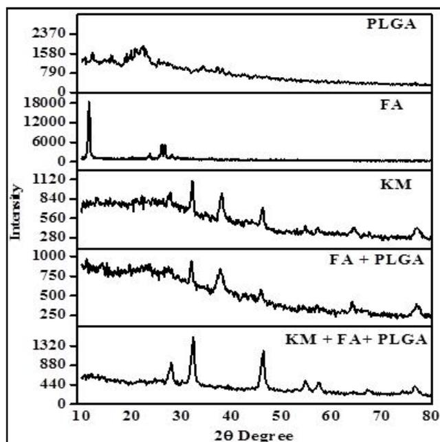
**Fig. 2.** XRD spectra of combinatorial nanoparticles, PLGA, FA (Folic acid), KM (Kaempferitrin), FA+PLGA and KM+FA+PLGA.
