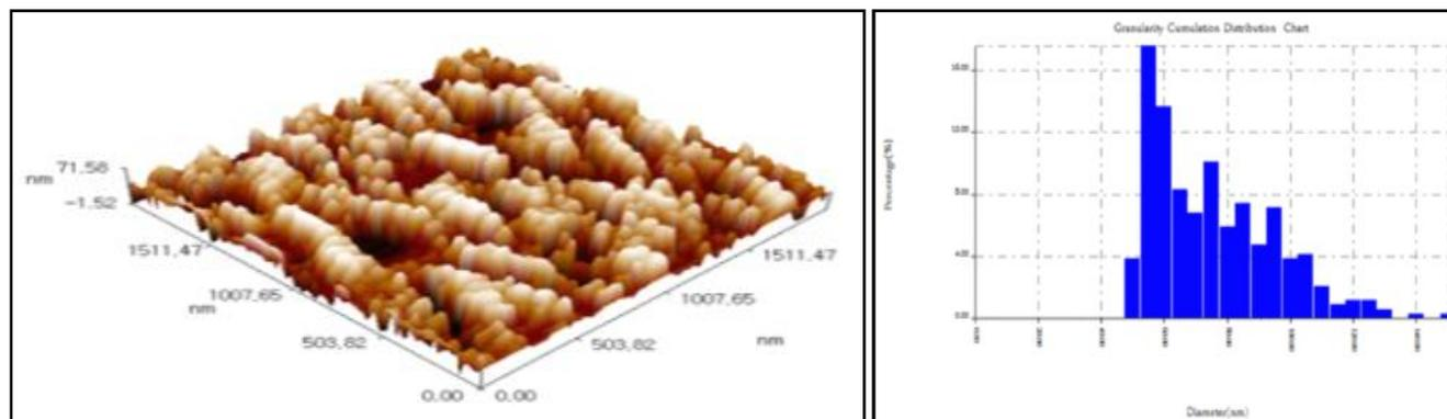
Fig. 1: Characteristics of  $\text{Fe}_3\text{O}_4$  NPs, spherical shape using AFM (right), granularity distribution chart (left).
