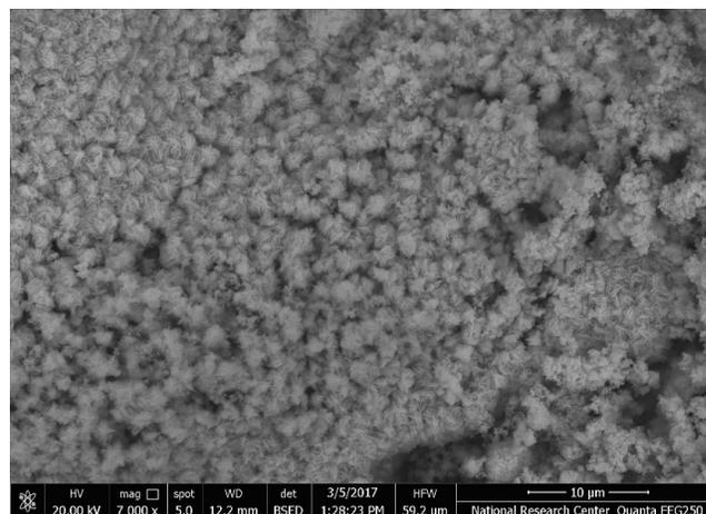
**Image 1:** Scanning electron microscopy image of Nano-ZincOxide.
