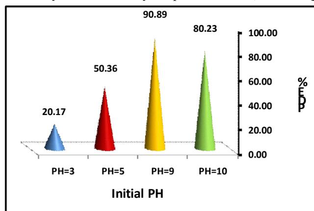
**Fig. 4:** Influence of initial pH on the photo degradation of malachite green dye. 50mg/L of dye and 0.16g of sensitized zinc oxide.
