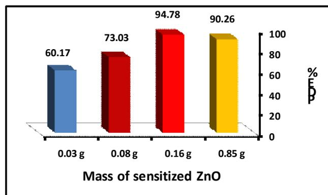
Fig. 2: Effect of sensitized zinc oxide mass on removal of malachite green dye, dye concentration is 50 mg/L.
