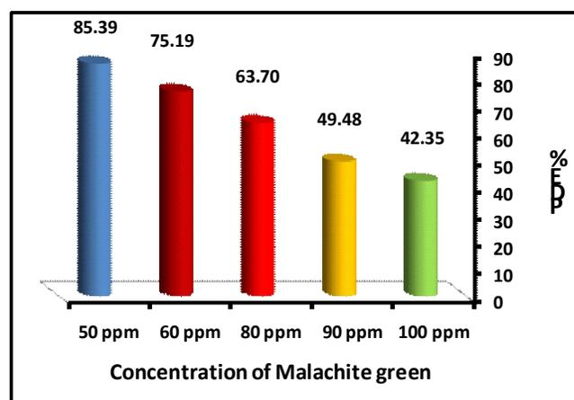
Fig. 3: Effect of malachite green stain concentration on photocatalytic process in the presence of 0.16g of sensitized zinc oxide.
