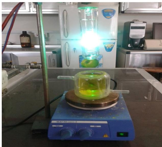
**Fig. 1:** Main compartments of the photocatalytic degradation cell used in removal of malachite green stain
