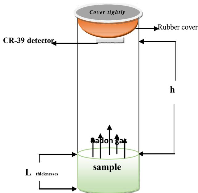
Fig. 1 : A schematic diagram of the sealed-cup technique.
