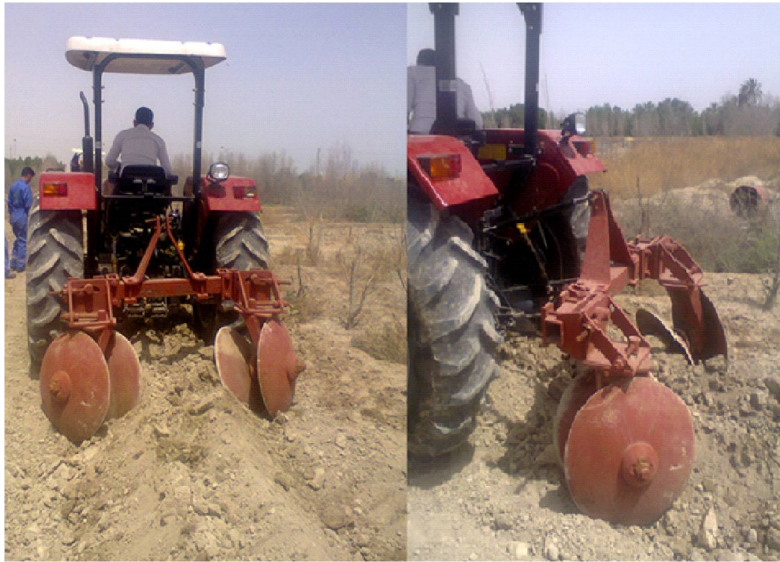
Fig. 1 : shows the connection of the dual disk ridge with the tractor.
