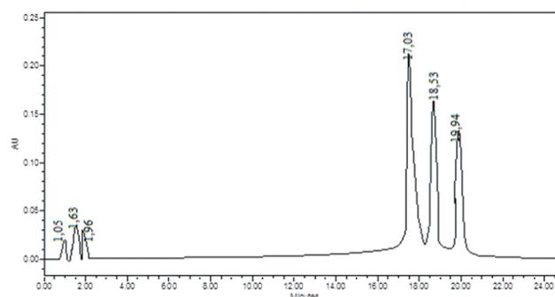
**Fig. 6 :** Chromatogram (zoom) recorded at 254 nm showing the phenolic compounds profiles identified and not identified of olive leaves (*Olea europaea* var. Sigiose).
