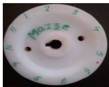
Fig. : A fabricated view of seed metering wheel of a manually operated multi-crop planter for showing corn seeds (Developed in SHUATS, Allahabad).
